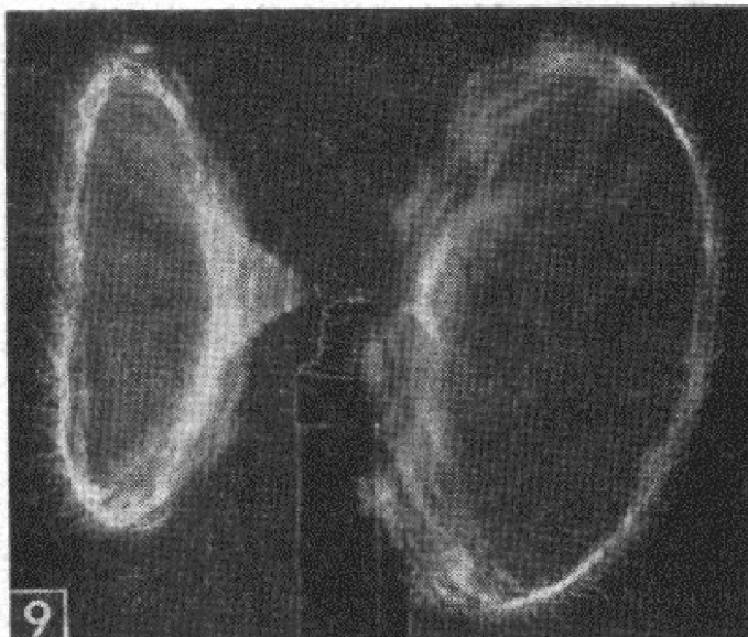
A 12 in. length of small nichrome or steel piano wire attached to the terminal at the center of the wire gives two blazing lavender colored rings of electrical fireworks.
